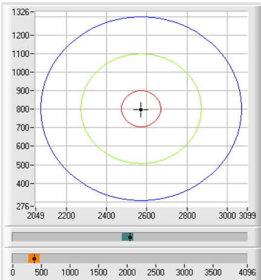
**Tip!** This mode is used if only one surface (vector) is taught, and this vector must be checked to avoid "drifting away". With the rising tolerance windows this can be detected very well, and countermeasures can be initiated, if necessary.
