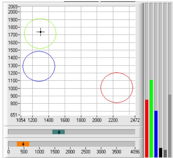
X/Y/INT GN or s/i/M GN: The panel that opens shows the taught X/Y/INT color spheres and the current gloss norm value GN. The current vector is shown as a black cursor. A three-side view with the graphs X/Y (s/i), X/INT (s/INT) and Y/INT (i/INT) was chosen for improved representation. The gloss norm value with the tolerance window set under No.: is displayed in a separate graph.
