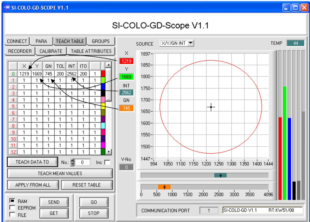
Now press the **SEND** button again to inform the sensor about the taught color. Then activate the **GO** mode again. When the sensor recognises a row vector, the corresponding row number is visualised on the software interface under **V-No.:** A value of 255 means that none of the taught vectors were recognised.
