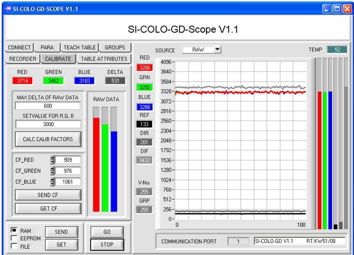
When the calibration factors have been calculated by the software on the user interface, they are automatically saved to the non-volatile EEPROM memory of the sensor. Calibration is then finished, work can then be continued in the main panel.
